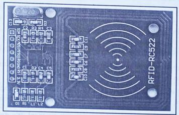
RFID has RC522 Arduino & Raspberry Pi compatible module that can be used to build an IOT based RFID application or application prototypes like attendance system.
