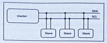
Here, two types wired lines i.e., Serial Data (SDA) and Serial Clock (SCL). Several slave devices can be connected to a master device using I2C.
