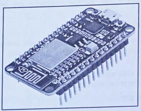
In terms of using the Wi-Fi protocol for IOT, there are some pros & cons to be considered. The infrastructure or device cost for Wi-Fi is low & deployment is easy but the power consumption is high, and the Wi-Fi range is quite moderate. So, the Wi-Fi may not be the best choice for all types of IOT applications, but it can be used for applications like Home Automation.
