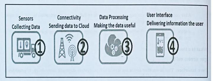
First, we collect data about the temperature and the location with our sensor devices (step 1). After that we use a network solution to send the data to a cloud service (step 2), where the data is transformed into useful information via data processing (step 3). Finally, the information is delivered to the end user via user interface (step 4).
