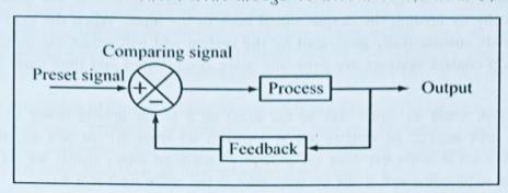
Feedback can be divided into positive and negative feedback. Positive feedback causes the new output to deviate from the present command status. For example, an amplifier is put next to a microphone, so the input volume will keep increasing, resulting in a very high output volume. Negative feedback directs the new output towards the present command status, to allow more sophisticated control. For example, a driver must steer continuously to keep his car on the right track.
