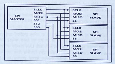
Here, slave devices have 4 connections i.e., SCLK (Serial Clock), MOSI (Master Output Slave Input), MISO (Master Input Slave Output), SS (Slave Select). First 3 pins share same line from controller but SS pin controls which slave device is active.
