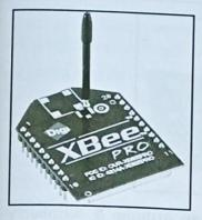
Having limitations related to data rate, range, and power consumption, Zigbee is only appropriate for Small-Scale Wireless applications. Though having some limitations, it provides a 128-bit AES encryption and is giving a big hand in making secure communication for Home automation & small Industrial applications. Zigbee too has its DIY module named XBee & XBee Pro which can be interfaced with Arduino or Raspberry Pi boards to make simple projects or application prototypes.
