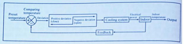
One advantage of using the closed loop control system is that it can adjust its output automatically by feeding the output signal back to the input. When the load changes, the error signals automatically generated by the system and will adjust the output. However, closed loop control systems are generally more complicated and thus more expensive to make.
